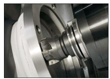
The EC-1600 and EC-1600ZT are equipped with a 7500-rpm geared-head 50-taper spindle that provides 340 ft-lb of torque for heavy cutting. For high-speed cutting, an 10,000-rpm geared-head spindle is available.
